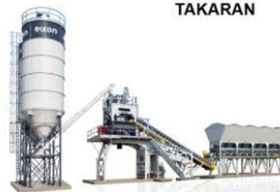
TIMBANGAN BATCHING PLANT
